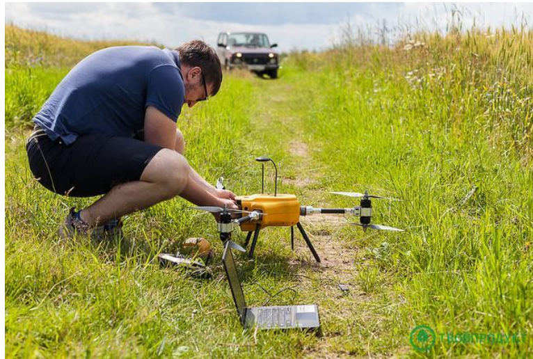
Figure 4. Field data collection with UAV and multispectral camera
